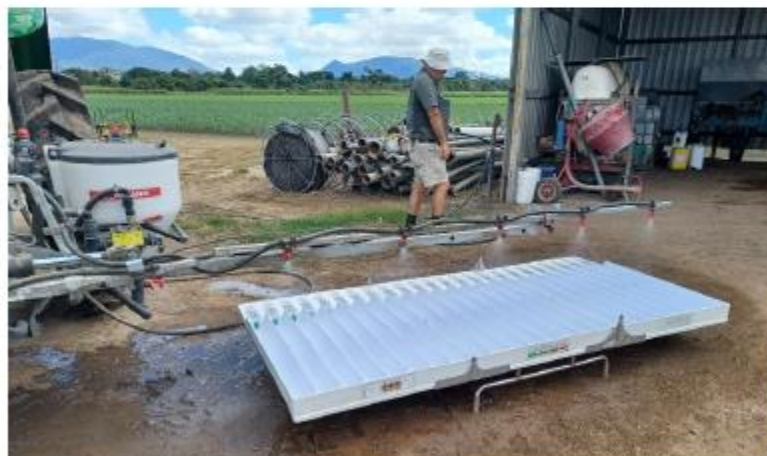
Figure 1: Patternator under spray boom catching droplets
